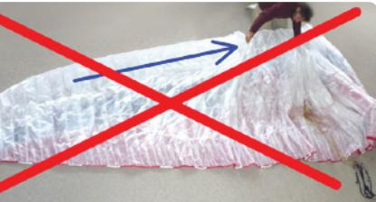
**IMPORTANT:** Do not fold the glider in the centre, you will bend the plastics, instead pack the wing with a full concertina method from tip to tip before packing into the stuff sac.
