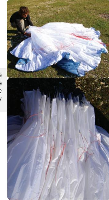
**Step 3.** Lay wing on its side and strap the LE. Note the glider is NOT folded in half, it is folded with a complete concertina from tip to tip. It is really important to not stress the middle cell or bend the plastics too tightly.
