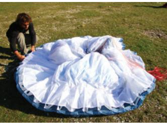
**Step 2.** Group the Leading Edge (LE) reinforcements with the A tabs aligned. Make sure the plastic reinforcements lay side by side.
