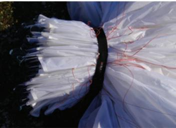
**Step 4.** Group together the middle/trailing edge of the wing by sorting the folds near the B, C and D tabs.
