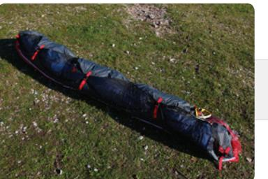
**Step 9.** Make the first fold just after the LE reinforcements. Do not fold the plastic reinforcements, use 3 or 4 folds around the LE.
